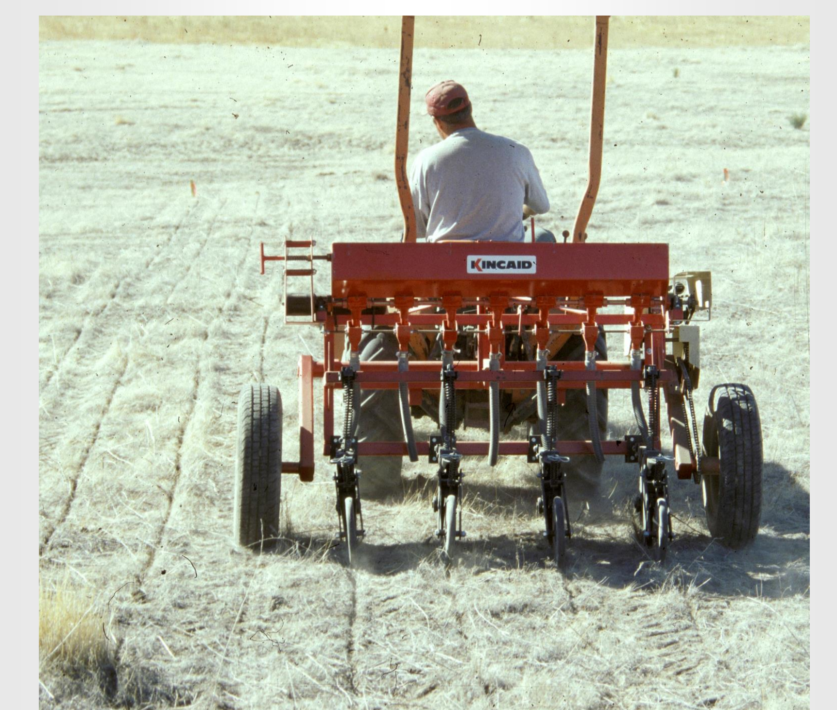
Figure 2. Seeding specific species using the kincaid no-till drill on herbicidal fallowed plot.
